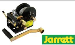
JARRETT HAND WINCHES - 10:5:1, 3 SPEED Heavy duty 800-1000kg capacity three speed winch ideally suited to large boats and general winching applications. Removable hex drive handle for quick ratio changes. Available with no cable, wire cable or web strap.
