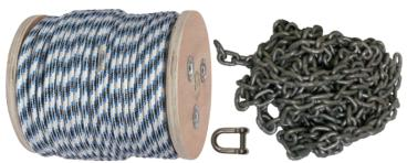
**DOUBLE BRAID ANCHOR ROPE & CHAIN KIT** High strength, flexible, low stretch double braid rope. Resistant to UV, oil,petrol, rot and mildew. Supplied with S/S thimble spliced onto one end, 6mm galvanised short link chain and a 6mm stainless steel slot head shackle. Reverse rolled for ease of putting onto anchor winches.
