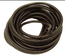
**SPLIT TUBING**Split corrugated conduit designed for quick, neat, cost effective wire harnessing or where neat, cost effective wire namessing or whet flexible protection is required for cable connections. The product is manufactured from black, flame retardant (UL94-V2), polypropylene copolymer, with a maximum operating temperature of 90°C. Available in 6 sizes.
