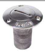
DECK FILLER - CAST S/S High quality heavy duty cast stainless steel deck fillers to suit 38mm hose. Supplied with safety chain, "O" ring seal and opening key. The name plate is cast into the filler in large print in two different types - PETROL or WATER.
